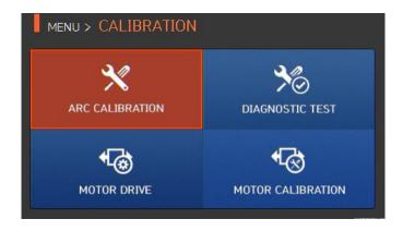
When executing arc calibration, arc voltage is automatically changed into a proper value. As this value is calculated by a certain computing program, a
